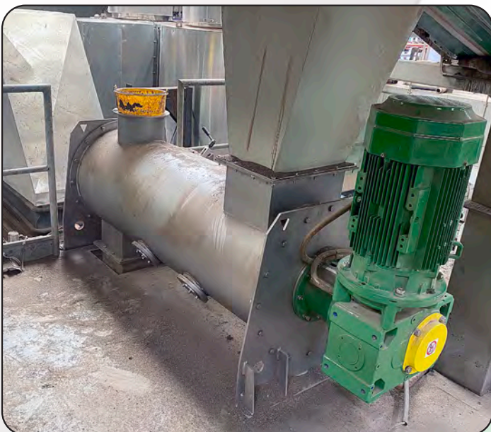
KCV mixer in 304SS for bio-fertilizers
