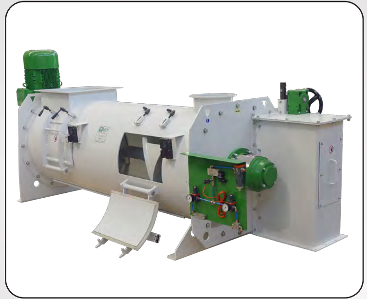
KCF continuous mixer in mild steel for food waste materials
