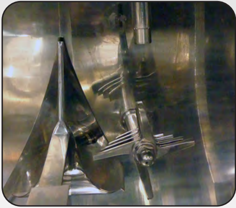
mirror polished 304SS plough, refiner blades and injection wand
